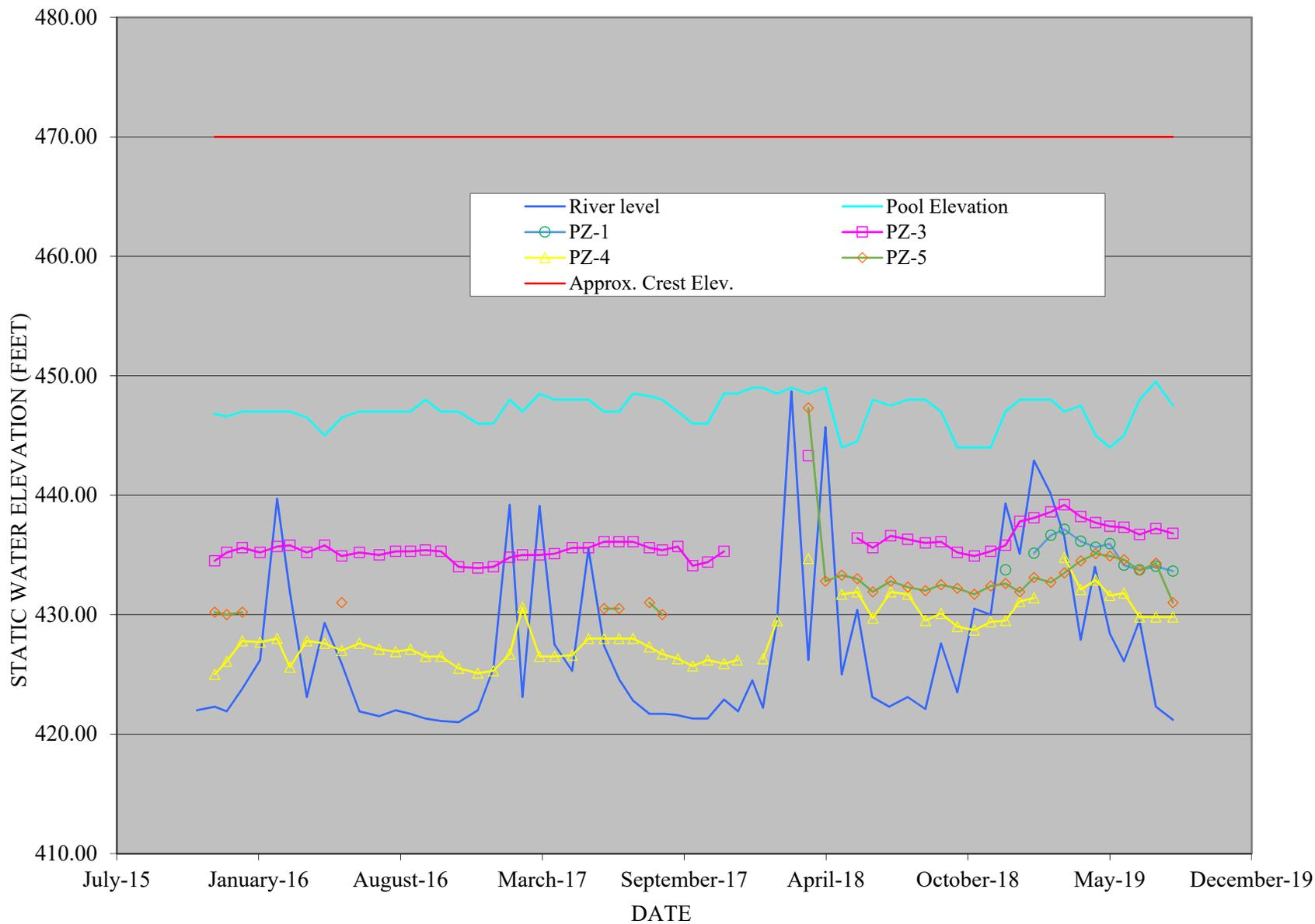
FIGURE 2. WEST BOILER SLAG POND PIEZOMETERS MEASUREMENTS
